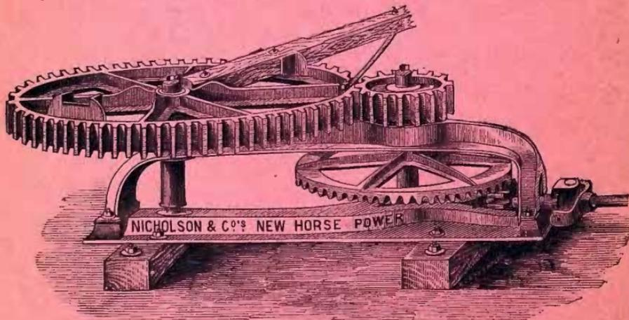
It is constructed entirely of Iron, and will be found to be simple in construction and very strong. The pole, or poles ("as it can be used either as a Single or Double Horse Power,") are fixed in such a manner that the pull is direct, the strain thus being reduced to a minimum. The speed is sufficient without the expense of an Intermediate Motion.
