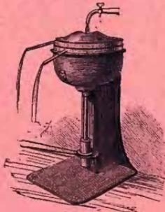
By using this Machine the Cream can be separated
