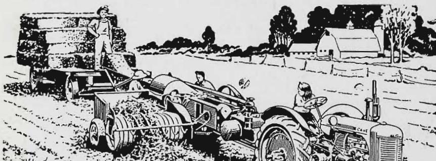
The Case Sliced Hay Pick-up Baler is capable of producing 2-1/2 bales per minute, 14 x 18 inches in size, weighing 60 to 75 lb. each. Its two operators can average 3½ to 5 tons per hour. It puts up the hay in ready-sliced bales for easy feeding and storage and saves the precious protein-rich leaves. Investigate these proved and practical balers at our Royal Show stand, or write for literature.
