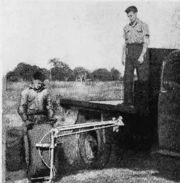
A comparative newcomer in the G-Well range, this Open Top Bag Loader is designed especially for the wheat farmer who transports unsewn bags between field and silo. The open top bag is placed on the platform at ground level—then the fast automatic action lifts the bag to truck height without spilling the contents. When the bag is removed the loading platform automatically returns to the ground.
