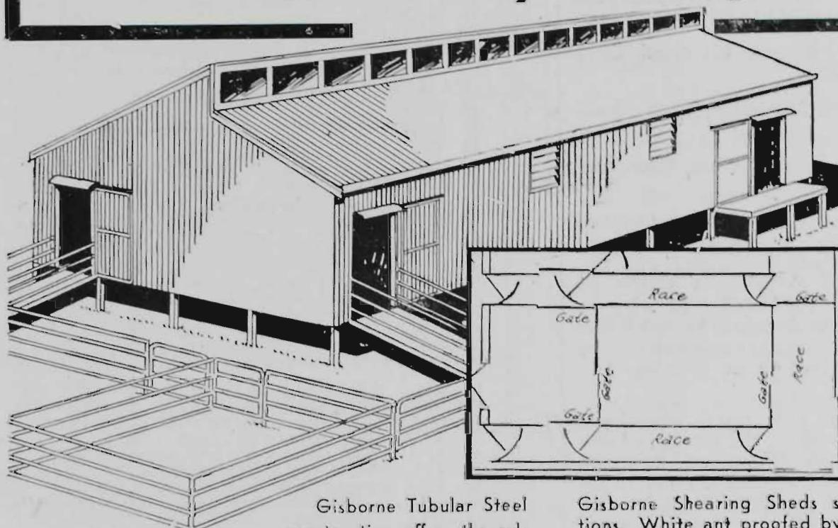
Gisborne Tubular Steel construction offers the advantage of complete flexibility. The hygienic steel structure and fittings and scientific overall arrangement permit smooth, speedy handling of sheep.
