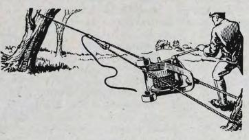
The machine is compact and sturdily built to deliver 260 times the power applied to the handle. It is quite portable and fitted with an automatic lowering gear, second speed, rope shortener, snatch block, etc. Ample cable to take an acre and a half from an anchor.
