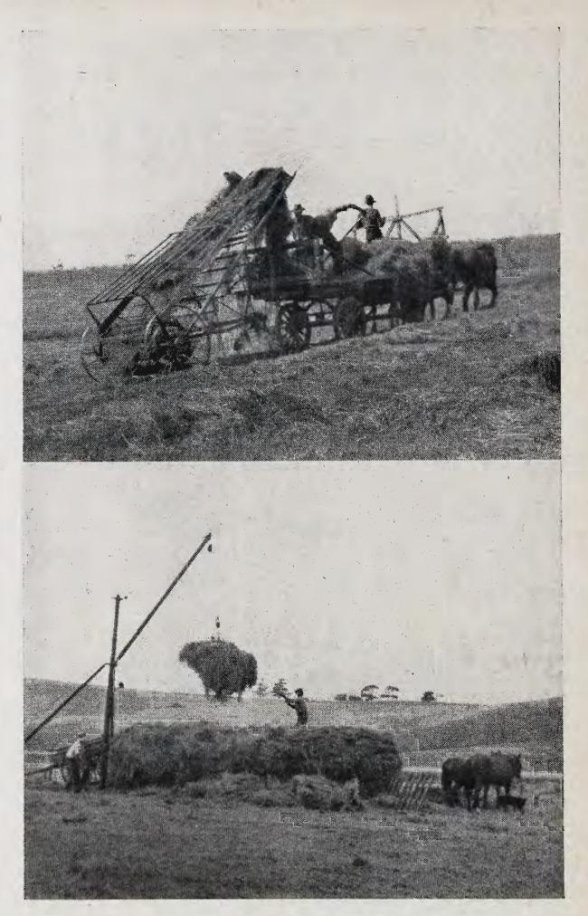
Above: Mechanical hay loader adapted for handling green material for silage.
