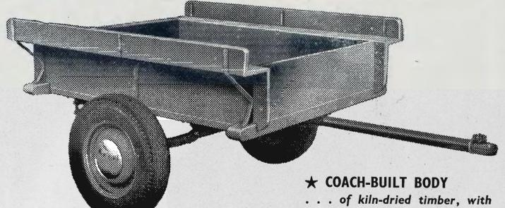
Available in limited numbers, the "Hendy" is the finest two wheel trailer on the road. Suitable for primary producers or any tradesman, the "Hendy", with its surprisingly large carrying space, will handle bulky and awkward loads of all types up to 15 cwt.
