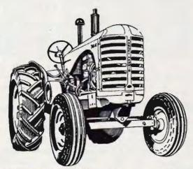
RELIABILITY— Produced with modern methods and equipment to the highest standards of British Engineering, the 744D is built throughout for a long working life. Its estimated horsepower, 29 drawbar, 36 belt, with maximum 39/42, gives ample power for general farm work. It has 6-cylinder smoothness, and all-day comfort for the driver on a "velvet-ride" hydraulic seat.
