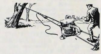
The machine is compact and sturdily built to deliver 260 times the power applied to the handle. It is quite portable and fitted with an automatic lowering gear, second speed, rope shortener, snatch block, etc. Ample cable to take an acre and a half from an anchor.
