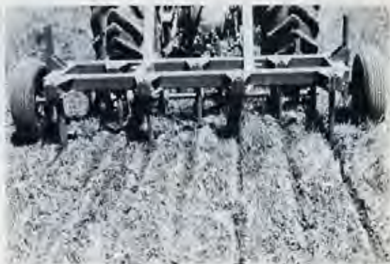
The Wallace Plough, showing how it moves through the soil, raising it and leaving a tent-like airduct that is capable of retaining moisture even months after the last good rainfall. This method of ploughing also appears to restrict the growth of weeds, and requires no superphosphate.
