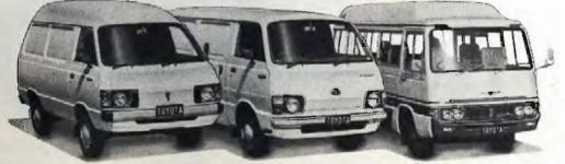
UTE ACE A pleasure to do business with. A great combination of work and play in a zippy 0.75 tonne van, cab chassis, steel back or deluxe van. Powered by an economical 1300cc engine. Also available with side windows. HIACE The Space Capsule. 2 litre or 1600cc, 4 cylinder engine. 58 litre fuel tank capacity. Tandem Master cylinder power assisted brakes. And a spacious interior of over 6 cubic metres (217 cubic teet) in the long wheelbase model.
