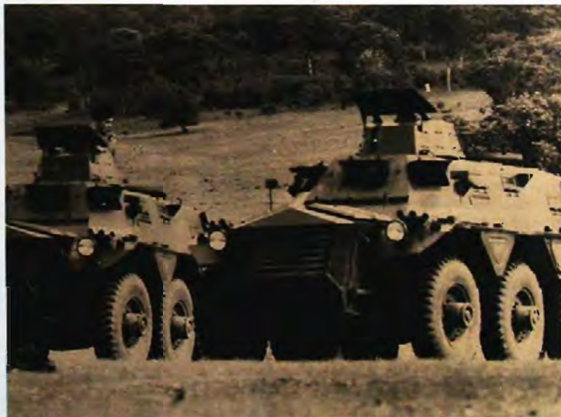
THESE SARACEN "CARS" WERE INTRODUCED TO THE AUSTRALIAN ARMY IN 1955. THEY WERE MADE IN ENGLAND AND COULD CARRY 10 COMBAT TROOPS INTO BATTLE AT A TOP SPEED OF 50 KM/H.
