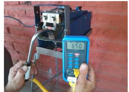
*Pyrometer indicating proper blade temperature of 650°C.*
